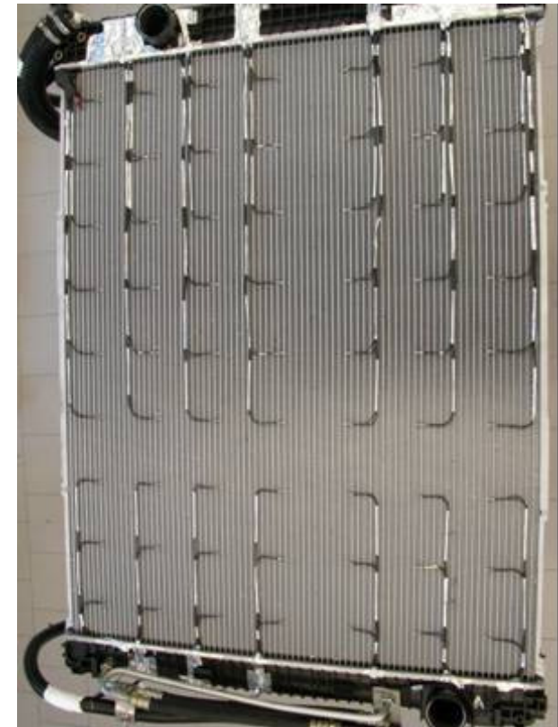
Radiator equipped with 63 Micro-Probes
